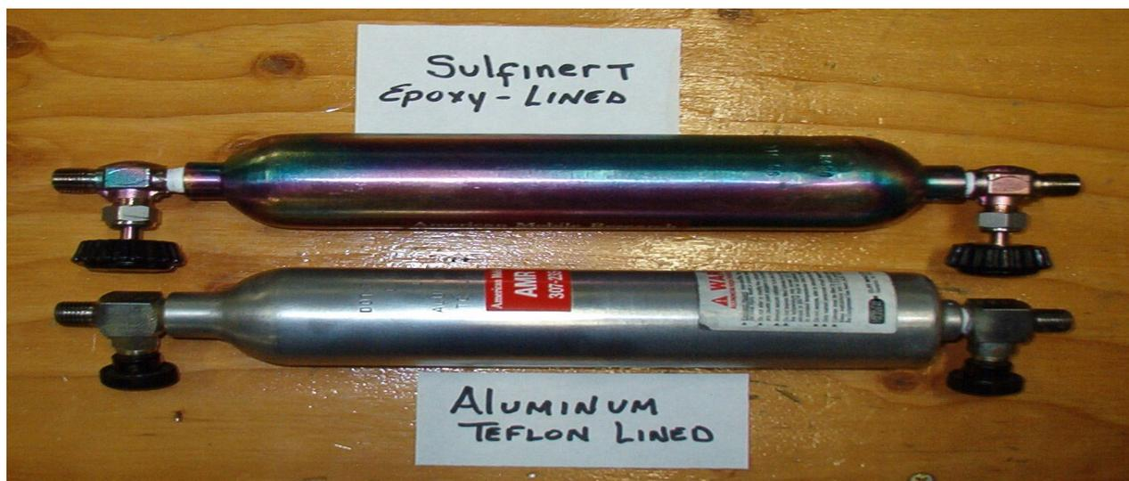
**[Fig.3] Chemically treated [lined] cylinders**
