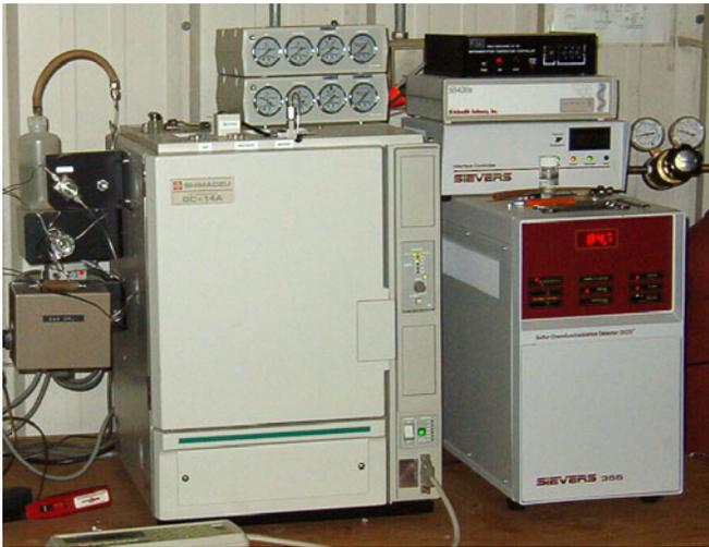
**[Fig.10] Sulfur chemiluminescence detector**
