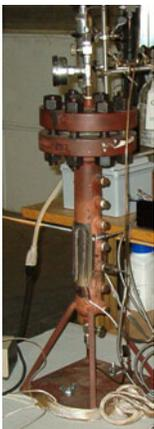
**[Fig.11] Absorbent test reactor**
