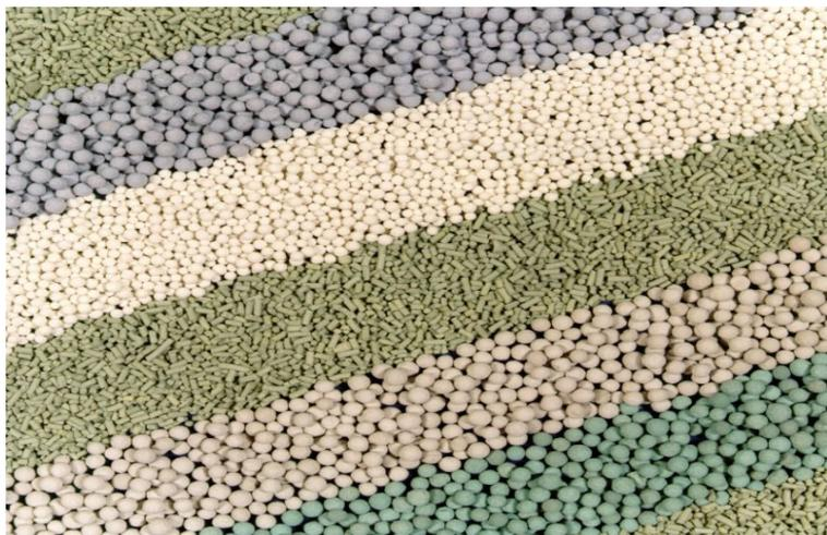
**[Fig.1] Mixed metal oxide absorbents for the low temperature desulfurization of NGL**
